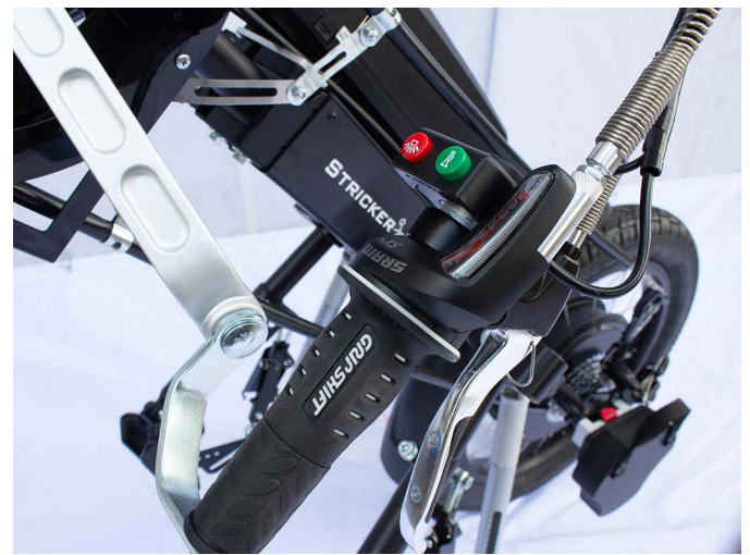
Fig. 20: Brake lever with brake contact and initiation of recuperation (interrupter contact is only connected to the right brake lever.)
