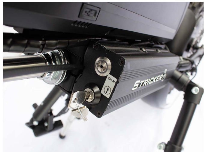
Fig. 12: Key switch on battery and control
