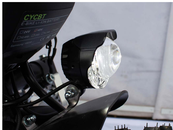
Fig. 18: Adjustment of the inclination of the lamp with integrated horn
