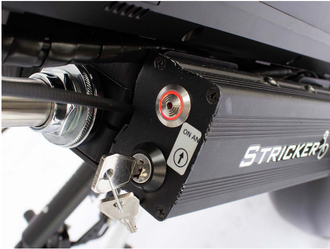
Fig. 19: The reverse light on the control lights up when reverse gear is activated
